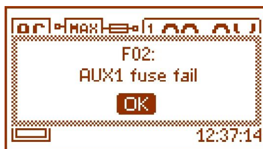
Fig. 18. Message indicating blown fuse at AUX1 output.
